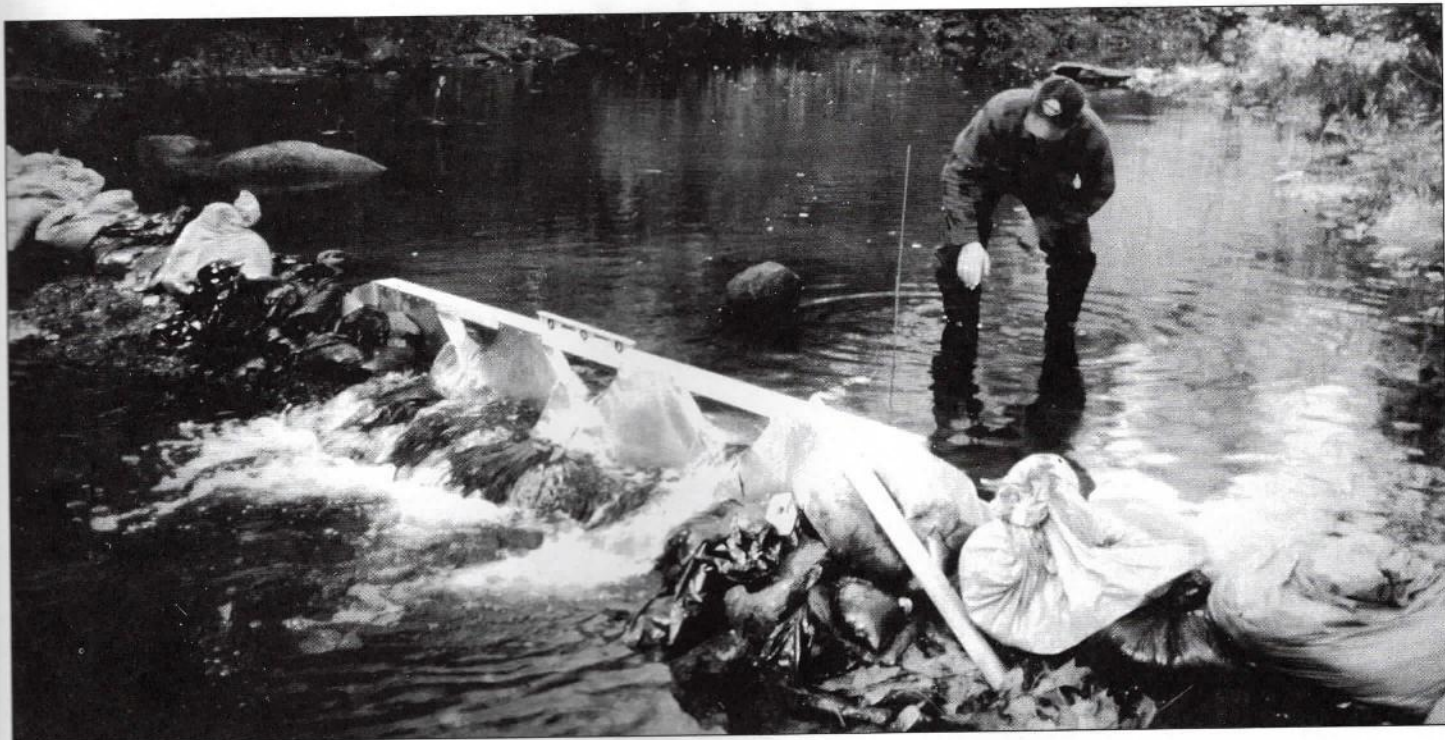
Temporary downstream weir measures Barcroft dam outflow to calibrate phosphorus monitoring computer system performance curve.
